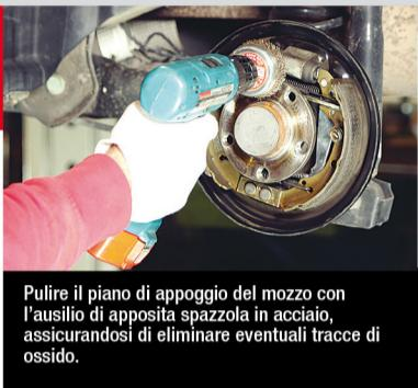
Clean the hub support surface using a special steel brush, making sure to remove any trace of oxide.
