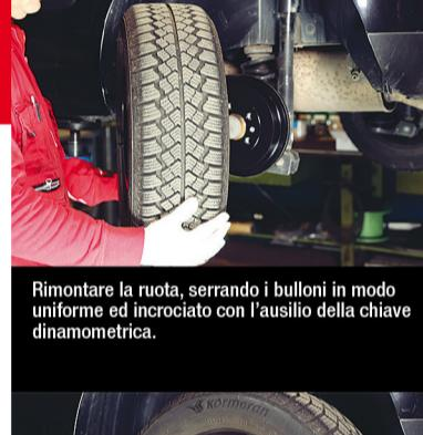
Remount the wheel, tightening the bolts evenly and crosswise using a torque wrench.
