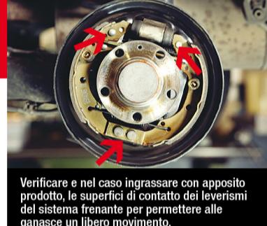
Check and if necessary grease the contact surfaces of the brake system levers using a special product to allow the brake shoes to move freely.
