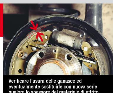
Check the wearing of the brake shoes and replace if necessary with a new series if the thickness of the friction material is less than the minimum prescribed by the vehicle manufacturer.
