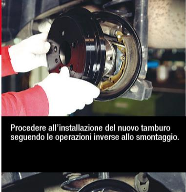
Install the new drum, following the instructions for removal in reverse order. If there is any trouble in fitting the drum into place, it may be necessary to use the brake shoe adjuster to close the shoes slightly (some vehicles also require an intervention on the handbrake adjuster).
