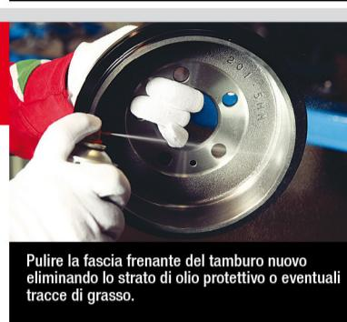
Clean the braking surface of the new drum, removing the layer of protective oil or any trace of grease.
