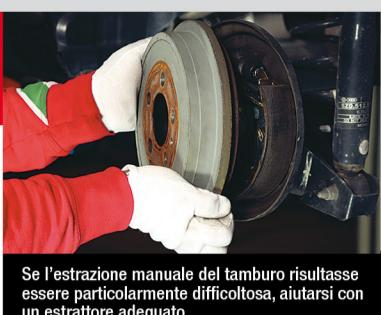
If manual removal of the drum proves particularly difficult, use a suitable extractor.
