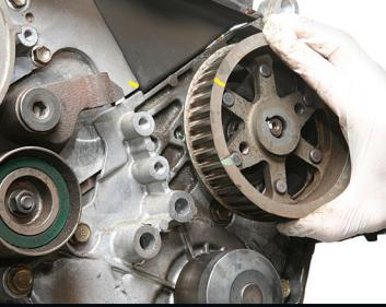
Dismantle the injection pump pulley if it is a single body combined with the water pump.
