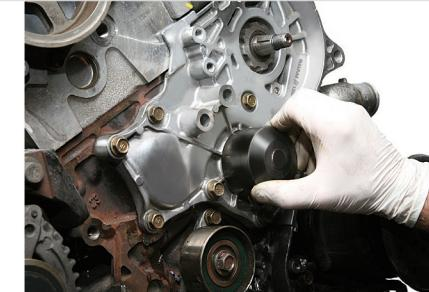
Make sure that the pump is centred and rotates freely, by turning the pump shaft with your hands.
