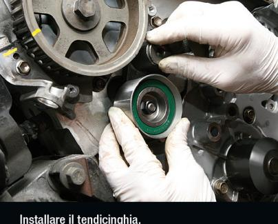
Install the belt tensioner, making sure that it operates correctly.
