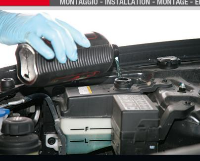
After you have vented the circuit, switch the motor off, wait for it to cool, and then check water level. Top up the circuit and close it.
