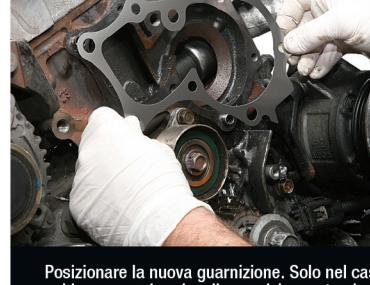
Position the new seal. Only if the pump has no seal, spread the adhesive between pump and motor block.
