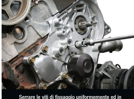
Tighten the securing screws uniformly and crosswise.
