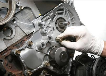
Turn the securing screws without tightening them.
