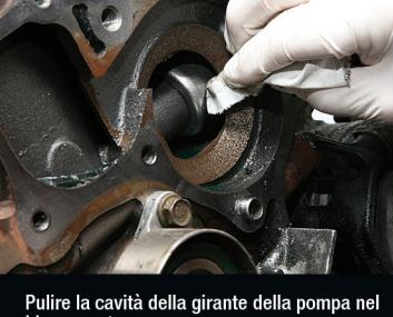
Clean the rotor cavity of the pump in the motor block.
