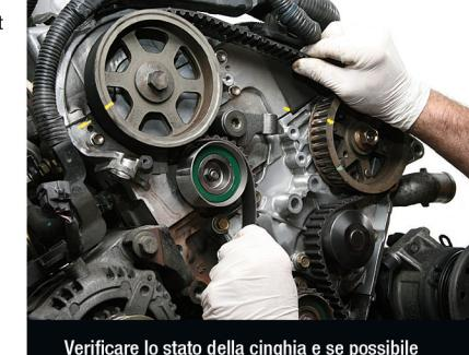
Check the condition of the belt and, if necessary, replace it by positioning it. At all times, when replacing the belt, make sure that the pulleys are positioned in line with the phase that you had marked.
